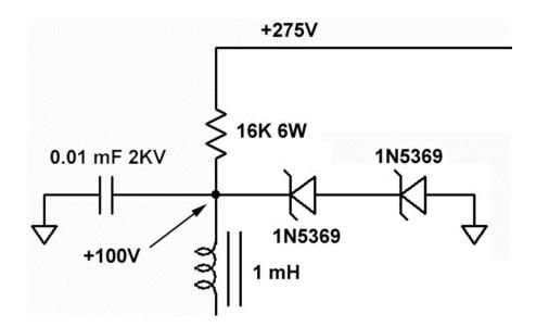
As a starting point for design, we need to know the working voltages 6 275V for the main B+ bus and 100V for the 6C4 plate in my case, and the operating current. When I first fired up the transmitter, the current draw for the oscillator was ~10 mA through the 3300 ohm plate resistor specified in the original design. The oscillator will draw less current at a lower plate voltage, so 10 mA seemed like a conservative design value.
